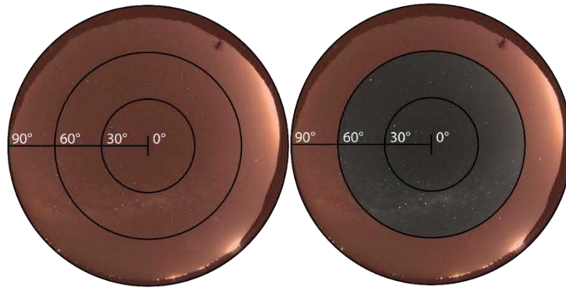
Figure 2: Measurement of mean pixel values; a. Whole-of-sky brightness (full image); b. Horizon brightness (60 – 90°). Shaded areas denote the region of the sky being measured.
